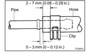
(d) Hose and tube connections are as shown in the illustra-
